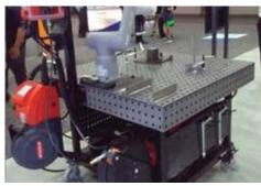
**Examples of cobot workstations for** welding applications.
